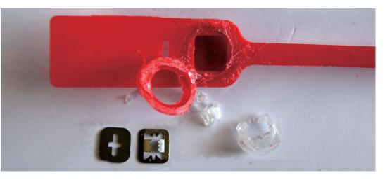
Double Metal lock mechanisms insert
