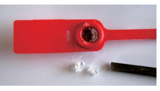
The cap is made with fragile material it is easy to be broken once prizing.
